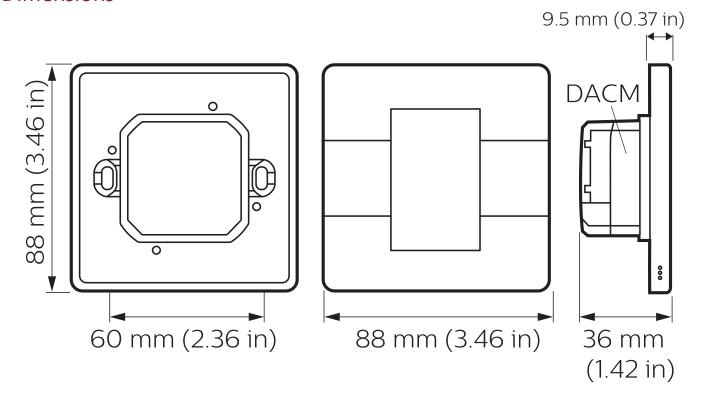
\* The mounting plate must be grounded to avoid field effect false triggering by nearby ungrounded metal objects.
