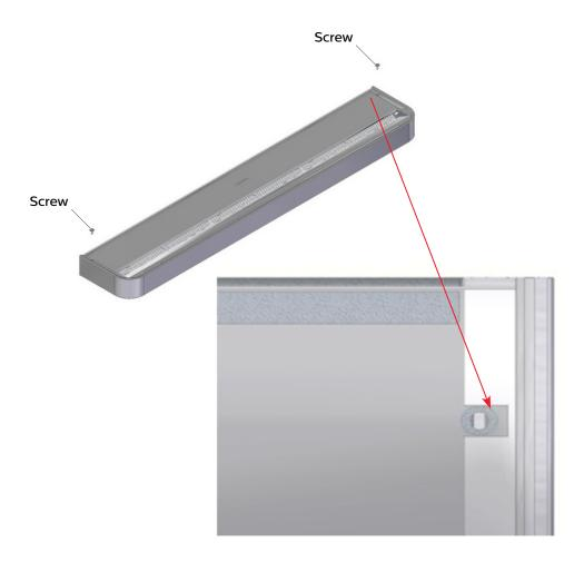
Fasten the light unit to the wall bracket with both supplied screws. These screws only need to prevent the luminaire from sliding back away from the wall and only need to be secured hand-tight. Maximum torque: 0.5 Nm
