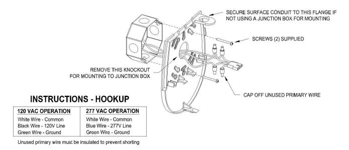
(2): If battery heater option has been ordered, installer must finish wiring heater according to installation voltage. All connections are to be made inside electronics module.
