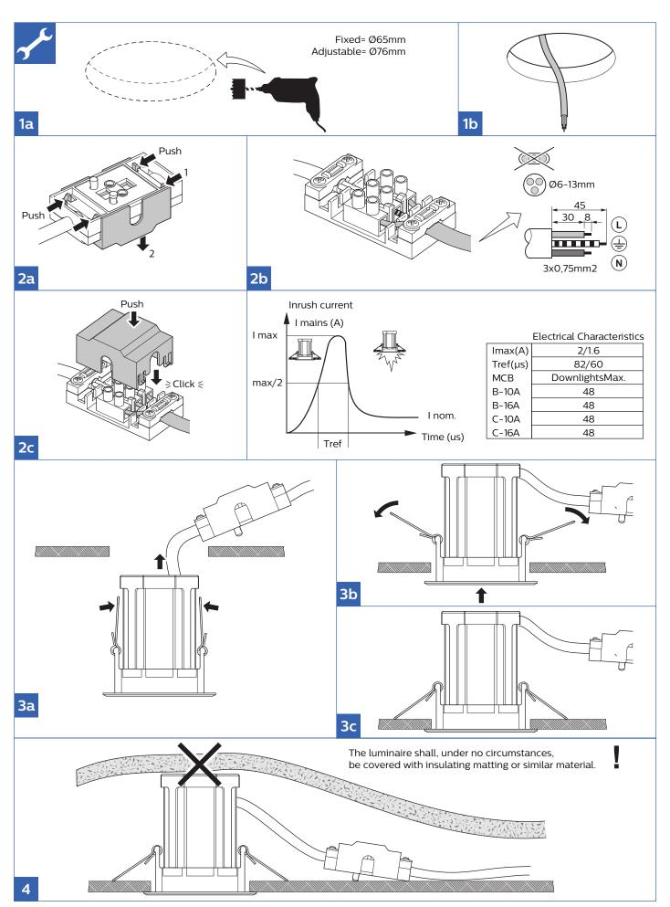
Only to be installed outside arms reach as recessed ceiling luminair. If the external flexible luminair cable or cord is damaged, it shall be exclusively repaired/replaced by the manufacturer or his service agent or a similar qualified person in order to avoid hazard. For complete and updated list of advised dimmers, please check the RS010 Spot page on the Philips Lighting eCatalog: http://www.ecat.lighting.philips.com
