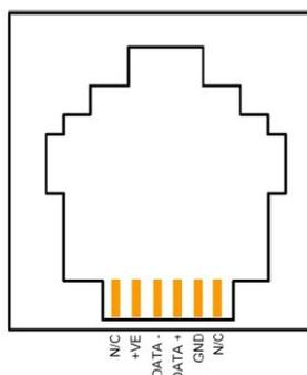
Serial Cable Permanent Connections
