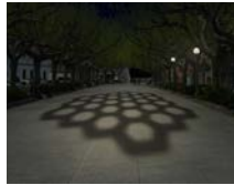
By adding ambient light (above, the luminaire on the right), the contrast of the projection on the floor is less and less good.
