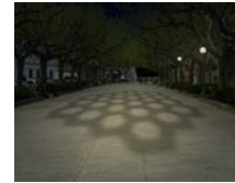
By adding ambient light (above, the luminaire on the right), the contrast of the projection on the floor is less and less good.
