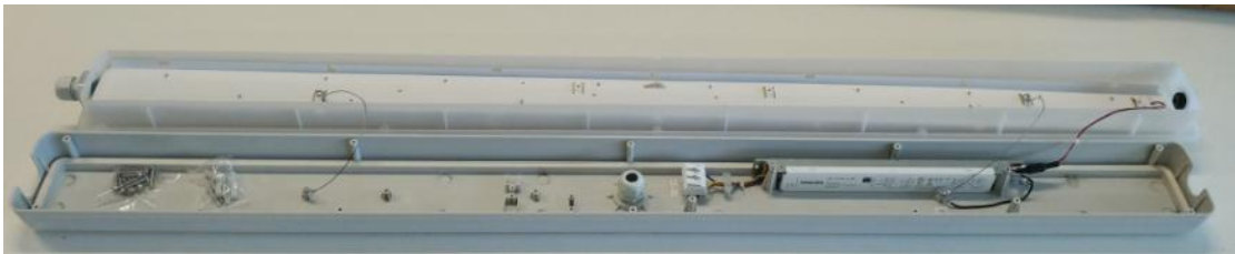
Open view of BCW098 LED20/NW PSU L600, BCW098 LED20/CW PSU L600
