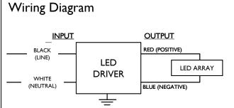
Input, Output and 0-10V Dimming use lead-wires. Lead-wires are 18AWG 105C/600V solid copper
