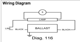
The wiring diagram that appears above is for the lamp type denoted by the asterisk  $(\sp{*})$
