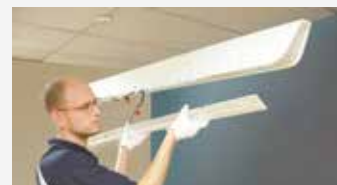
3. Remove the LED assembly.
