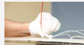
4. Disconnect the LED quick-wire plugs.
