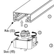
Put track adaptor into track align track adaptor slot to track rib 注意槽口装配方向. (轨道接
