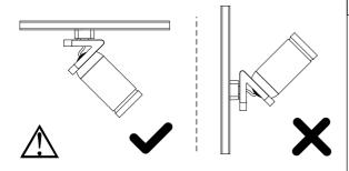
Luminaire recommend to be used with Track on the ceiling. Lifetime might be influenced when projector is pointed upwards. 推荐使用吸顶式的轨道(灯具出光方向朝下)。当灯具出光方向朝上时,灯具寿命可能会受到影响。
