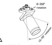
Please adjust the light direction when the power is off. 请在未通电时调节灯具照射角度。
