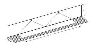
Meets Life Safety Code standard minimum illuminance of 0.1 FC and average illuminance of 1.0 FC. Indoor performance based on 80/50/20reflectance and assumes open space with no obstructions. Refer to  $% \left\{ 1,2,\ldots ,n\right\} =0$ charts for mounting height. Add 1' to mounting height for ceiling height. Outdoor performance based on 0/30/10 reflectance. Analysis based on independently tested photometrics.
