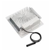
On Mini 300 LED gen2 luminaires, radial heatsink fins increase air velocity through the convective cooling system, effectively radiating heat out and away from the luminaire.
