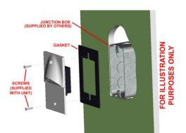
This product is designed for installation into new construction or retrofit applications. For new construction, no preparation is required other than making sure a single gang junction box or 4S/5S junction box with metal mudplate is installed and power is supplied. For retrofit applications, removal of the electrical outlet, switch or existing equipment must be done first by a certified electrician.
