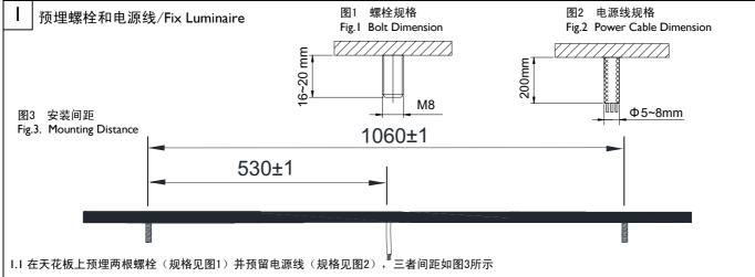
1.1 Embed two bolts(SPEC refer to Fig.1) and power cable(SPEC refer to Fig.2). The mounting distances between them refer to Fig.3
