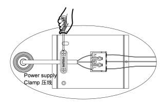
Power supply Connection 电源线连接
