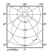
Light Distribution Diagram - DN027B LED6/CW D90 RD
