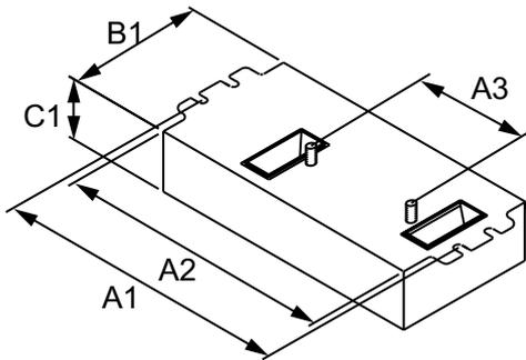
ELE BALLAST (2) 26W CFL (4-PIN) 120-277V
