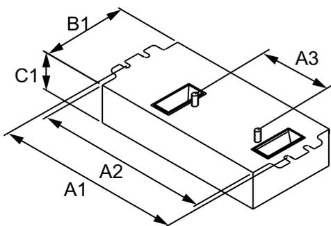
ELE DIM BALLAST (1) 18W CFL (4-PIN) 120V
