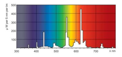
Spectral Power Distribution Colour - 54W/830 Min Bipin T5 HO ALTO UNP
