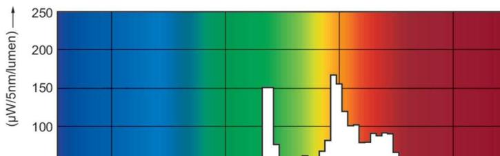
Spectral Power Distribution Colour - MC CDM-Tm Elite Mini 50W/930 GU6.5
