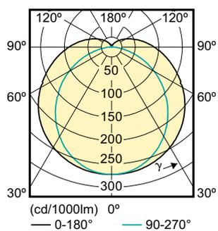
Light Distribution Diagram - MAS LEDtube VLE 600mm 10W830 T8C ROT
