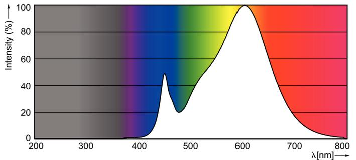
Light Distribution Diagram - MAS LEDtube 600mm 9W 830 T8 RS
