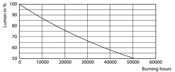
Lumen Maintenance Diagram - MAS LED spot ND 41W PAR30L E27 830 30D
