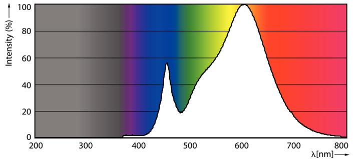
Spectral Power Distribution Colour - MAS LED spot ND 41W PAR30L E27 830 30D
