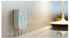
The Hue Bridge is an essential component to a personal Philips Hue smart lighting system. It is the brains of the operation, communicating with both your smart light bulbs and the Hue app to ensure that everything works together. It also enables smart home automation features like scheduling routines and timers.
