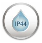
This Philips outdoor light is especially designed for humid outdoor environments. It was tested rigorously to ensure its water resistance. The IP level is described by two figures: the first one refers to the protection level against dust, the second against water. This outdoor light is designed with IP44: it is protected against splashing water, this product is most common and ideal for general outdoor use.
