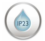
This Philips outdoor light is especially designed for humid outdoor environments. It was tested rigorously to ensure its water resistance. The IP level is described by two figures: the first one refers to the protection level against dust, the second against water. This outdoor light is designed with IP23: it is protected against spraying water and ideal for lighting a veranda or a porch.
