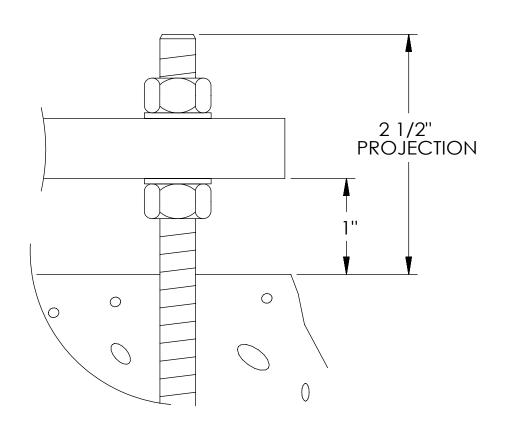
MOUNTING TEMPLATE FOR: RF6, RD6, RL72, RB71, RR70, SL8, SL7, SL6, AB06, AB04, AB14, AB03, AB15, LL-301, LL-300
