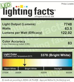
Photometric Testing of Solid-State Lighting. The U.S. Department of Energy (DOE) verifies product test data and results.
