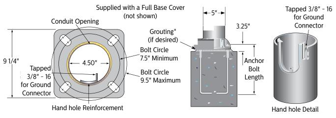
\* Grouting should include a drainage slot or tube (by others) to permit water to drain from the base of the pole. Failure to provide drainage may weaken the pole base structure over time and may result in pole base failure, for which Gardco is not responsible.
