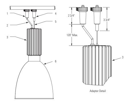
Typical complete installation shown (Power Head and Reflector must be ordered separately).
