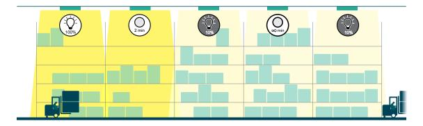
This mode is relevant for warehouse environments that are constantly occupied throughout the day or for spaces that require lights to stay at a dimmed level instead of shutting off when unoccupied.
