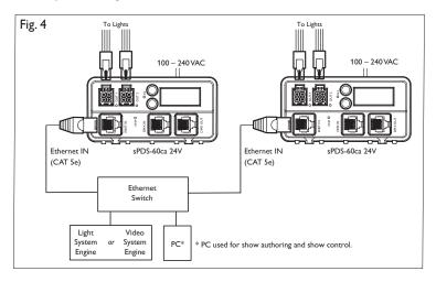
Connect the CAT-5e data cable, with RJ45 connectors on both ends, to the Ethernet switch and to the ENET IN port on the sPDS-60ca 24V power/data supply.
