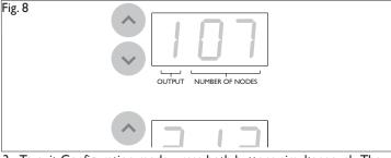
To exit Configuration mode, press both buttons simultaneously. The base address for sPDS-60ca 24V will appear on the display.
