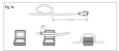
Connect the IEC power cable to the back of sPDS-60ca 24V. Plug the IEC power cable into a standard 100 – 240 VAC outlet. Tighten the screw to secure the clamp. (See Fig. 5b.)
