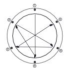
Use several rotations of the following sequence to firmly tighten the lens ring screws, to 25 in/lbs.
