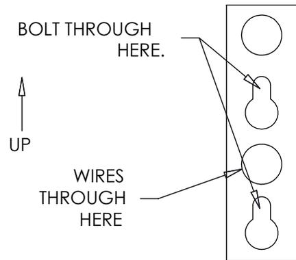
ORIENT MOUNTING PLATE AS SHOWN. MOUNTING BOLTS ARE TO GO THROUGH KEY-SLOTS.
