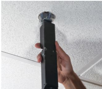
Insert fixture through 2 1/8" cutout in ceiling. 2 1/8" is standard hole saw size. Hinged design requires only 5 1/2" plenum depth (Non-IC).
