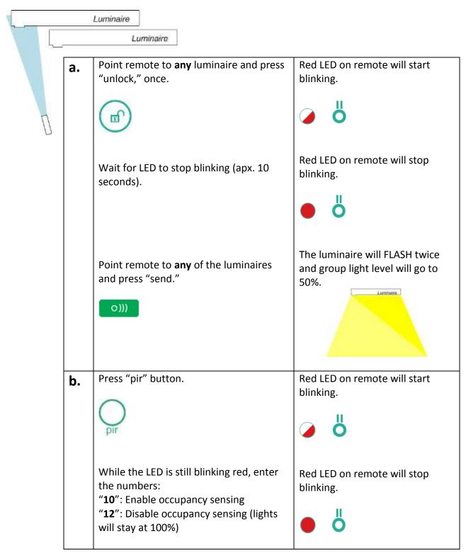
Point to the luminaire that needs to be The luminaire will FLASH twice altered, press "send." and group light level will go to 50%. 0))) Repeat step "b" for all the luminaires that need to be reconfigured. Point to any of the luminaires in the Red LED on remote will start group and press "lock." blinking. The luminaire will FLASH twice. Wait for LED to stop blinking (apx. 10 Group is ready for normal seconds) then press "send." operation. 0)))
