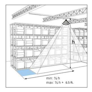
When configuring industrial spaces with SpaceWise Remote, large groups of 30-50 luminaires are recommended to maintain the lighting aesthetics of the space and improve reliability of the system. Smaller groups may turn off more frequently than desired.
