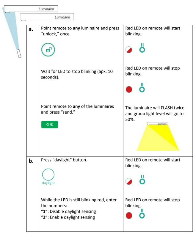
Point to the luminaire that needs to be The luminaire will FLASH twice altered, press "send." and group light level will go to 50%. 0))) Repeat step "b" for all the luminaires that need to be reconfigured. Point to any of the luminaires in the Red LED on remote will start group and press "lock." blinking. The luminaire will FLASH twice. Wait for LED to stop blinking (apx. 10 Group is ready for normal seconds) then press "send." operation. 0)))
