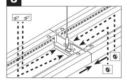
SLIDE MODULES TOGETHER: Secure joint from above using supplied nut and bolt hardware.
