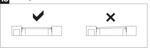
Identify smooth side of the Light Guide and ensure it is installed smooth side DOWN. Install Light Guide panel into LED fixture after joining and wiring is complete. Ensure panel is seated correctly as shown above.
