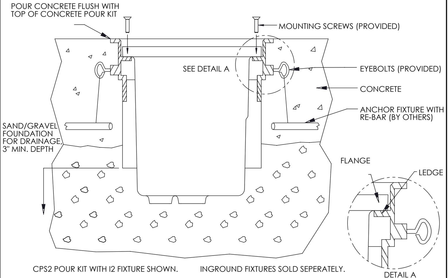
ATTENTION: CONCRETE POUR KIT MUST BE INSTALLED IN CONJUNCTION WITH FIXTURE HOUSING.
