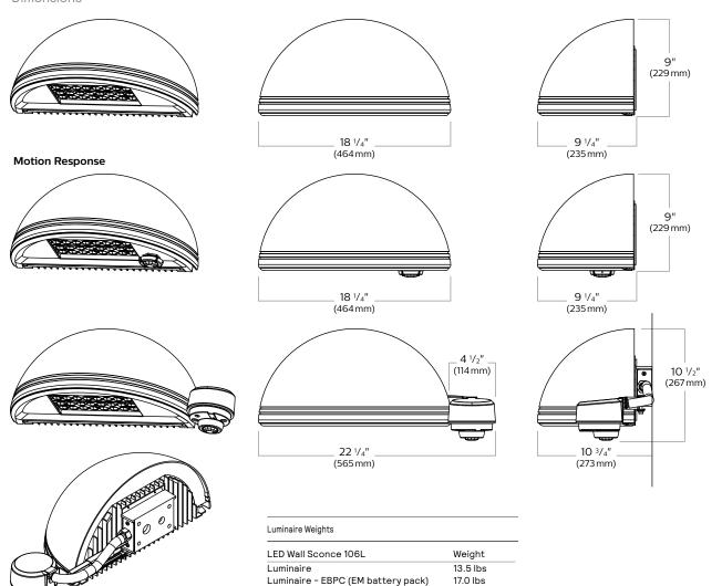
Luminaire - Integrated system controls 16.3 lbs
