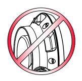
Do not loosen sealing bolts 请勿拧松密封螺栓
