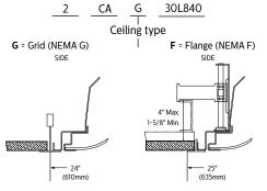
Luminaire end Access plate location 7/8" dia hole Open with screwdriver and bend to 90° and Grid tees (by others) 7/8" dia. K.O
