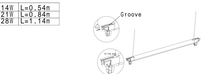
Slide the suspension mounting device into the groove, till the end. (Preferably pre-connect the batten/battens in case of suspension mounting.) \* Not provided as accessory.
