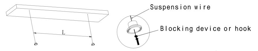
Insert appropriate suspension wire(with blocking device)<sup>\*</sup> through the suspension mounting device and firmly fix the same on the ceiling. Repeat above step for the second wire, at a distance as given below:
