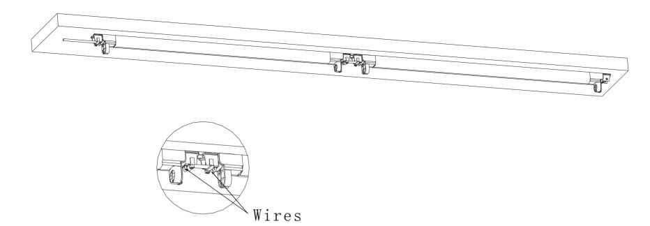
C). Connect two terminal blocks together by short wires, and fix the clamps tightly.
