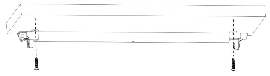
Twist off the screws and take off the batten.
