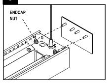
Attach endcap to first and last module in each row using 11/32" NUT DRIVER OR supplied hardware. WRENCH REQUIRED.
