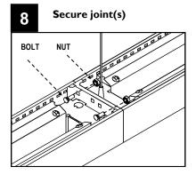
SLIDE MODULES TOGETHER: Secure joint from above using supplied bolts & nuts.
