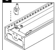
Fold rectangular flaps in wire cover and insert the A/C mounting bracket through the top. Raise bracket until security tab is engaged.
