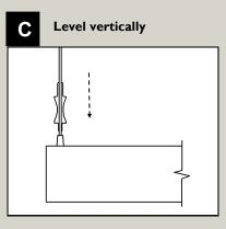
LEVEL VERTICALLY: Support fixture from below and use supplied cable gripper
