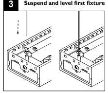
With two people, raise the first fixture to the ceiling. At each end of the module, insert aircraft cable into cable adjuster. The adjuster will automatically grip and hold the cable. Do not force cable into adjuster. See instruction
