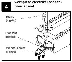
NON-POWER LOCATIONS: Cap all wires and tuck into wire cavity.
