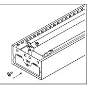
Attach brackets to fixture using supplied fasteners.
