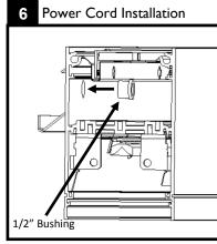
Determine power feed location on fixture. Attach supplied 1/2" bushing as shown.
