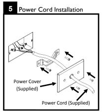
Complete wall power connections and attach supplied power cord through power cover. Attach cover to utility box.
