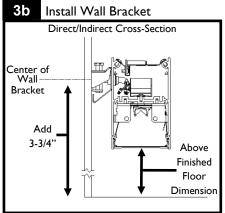
Determine above finished floor dimension and add 3-3/4" for direct/indirect configuration. Draw center line, level and center wall brackets. Install to structure using appropriate hardware (by others).
