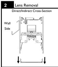
Remove lens from fixture and set aside until fixture installation is complete. Use cotton gloves to handle lenses and keep in a clean environment.
