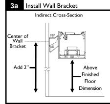
Determine above finished floor dimension and add 2" for indirect configuration. Draw center line, level and center wall brackets. Install to structure using appropriate hardware (by others).
