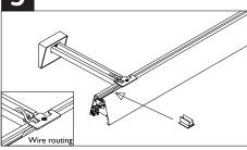
Run power cable in fixture channel and through power plate at the end of the fixture. Secure power cable into fixture channel using supplied cable clips at 4" increments.
