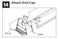
Snap gasket to the end of the fixture and attach end caps using supplied #8 screws.
