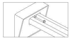
Slide on Wall covers and use supplied #8 lock-nut to secure to cantilever arm bracket, (non-power mount shown).
