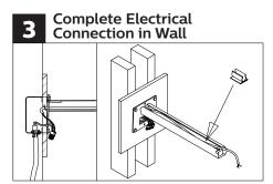
(Power locations only) Feed power cable through 1/2" hole in mounting bracket. Complete electrical connection to junction box through square cut out in mounting bracket. Use supplied cable clips to secure the power cable to the interior of the mounting channel at 4" increments.
