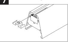
Attach the Fixture to the Bracket
