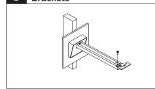
Attach fixture mount brackets to cantilever arm brackets using supplied 1/2"-20 bolts. Do not fully tighten.
