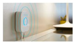
The Hue Bridge is an essential component to a personal Philips Hue smart lighting system. It is the brains of the operation, communicating with both your smart light lamps and the Hue app to ensure that everything works together. It also enables smart home automation features like scheduling routines and timers.
