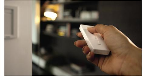
With the battery-powered dimmer switch, you can control up to 10 smart lights simultaneously. The switch — which can be removed from its wall mount and used as a remote control — allows you to dim and brighten your lights or cycle through four preset light recipes
