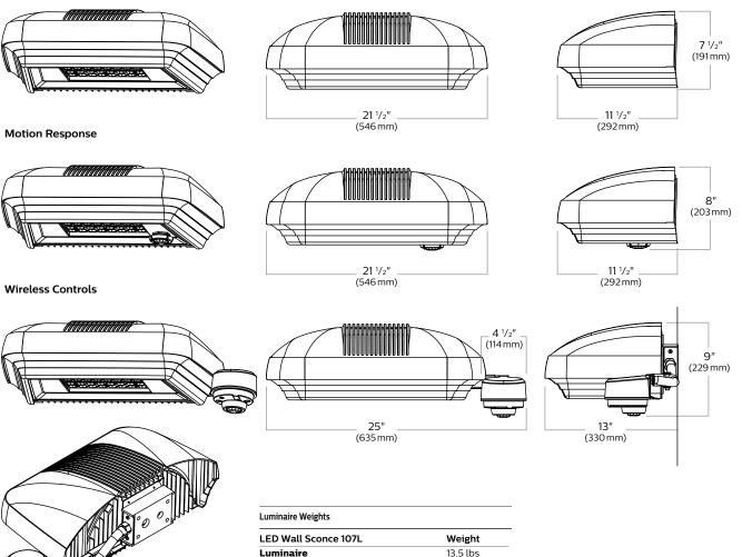
Luminaire13.5 lbsLuminaire - EBPC (EM battery pack)17.0 lbsLuminaire - Integrated system controls16.3 lbs
