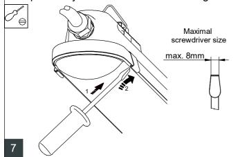
Do not touch electronic components! Electronic components maybe under high voltage. Caution, risk of electric shock!
