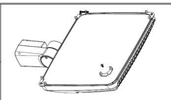
ATTACH BARN DOORS USING (QTY 8 – 2 PER DOOR) 1.5" SCREWS PROVIDED. SCREW WILL ENTER FROM THE OUTSIDE OF THE BARN DOOR AND ENGAGE MOUNTING BRACKET. SIDE DOORS ARE IDENTICAL, TOP AND BOTTOM DOORS ARE DIFFERENT. TOP DOOR CLEARANCE SLOTS FOR MOUNTING BRACKET WILL BE CLOSER TOGETHER THAN THOSE OF BOTTOM DOOR.
