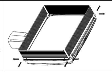
ONCE DOORS HAVE BEEN ATTACHED TIGHTEN 3/8" BRACKET SCREWS TO SECURE MOUNTING BRACKETS TO HOUSING.
